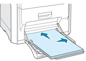
4 Pinch the paper width guide and slide it to the right to touch lightly against the edge of the material without bending it.
